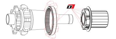
Free Hub Installation on Hub Shell Apply a few drops of Dumonde Tech Freehub Oil to the drivering, pawls, and freehub seal, as well as a thin film of grease to the axle.
