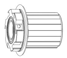
Inner Freehub Bearing Removal - Once the drive components are removed from the freehub shell there will be 1 inboard and 1 or 2 outboard bearings (depending on the freehub type) with a cylindrical spacer between them.
