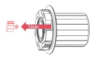
Freehub Disassembly + Service - Freehub drive components are easily removed by hand. The pawls slide out of the pawl pockets. The pawl springs should be paid special attention to when removing the pawls as to not lose them. The spring will typically slide out with the pawl.
