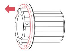
Freehub Seal Access - This step is typically unnecessary in most service situations. Once the pawls are removed you can then access and service the freehub seal if needed. The freehub seal can be lifted from its seat with a little pressure.
