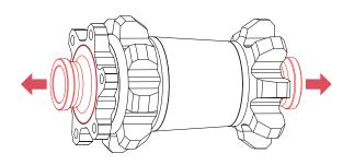
Front Hub Disassembly - The front hub consists of a cylindrical axle spacer held in place by two bearings and two endcaps pressed onto each side.
