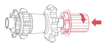
Once the freehub makes contact with the drivering gently press the **freehub** onto the hub while twisting it counter-clockwise to engage the pawls into the drivering.
