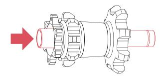
After the non-drive side bearing has been pressed in, put another thin film of grease on the outside the hubs axle, then insert it through the non-drive side of the hub.
