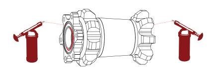
Front Endcap Installation - Coat the seal of the bearing with a film of marine grease before pressing the endcaps into the hub.
