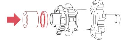
Press the non-drive side bearing over the end of the axle, into the non-drive side of the hubshell.
