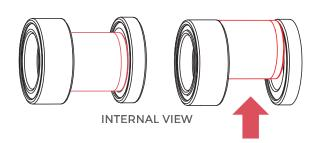
The cylindrical spacer can be shifted out of the way to access the inner race. Careful removal of one of these bearings (the order doesn't matter) with a blind bearing puller or tapped out with a drift or a punch will remove the bearing, allowing the spacer to be withdrawn. The remaining bearing should be removed in the same manner.
