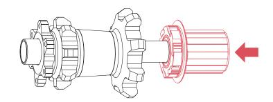
Push the freehub onto the axle. Be sure that the freehub's inner spacer is centered, then slide the freehub over the axle onto the rear hub's drive side.
