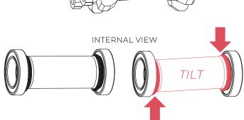
Front Hub Bearing Removal - With the hub's end caps removed, there will be two bearings on each side with a spacer held captive in between them.
