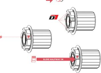
Freehub Pawl Installation -Lubricate the pawl-pockets with Dumonde Tech Freehub Oil. Take a pawl spring and push it into the spring-hole in the freehub body. A small Allen wrench will help locate the spring into the bore.
