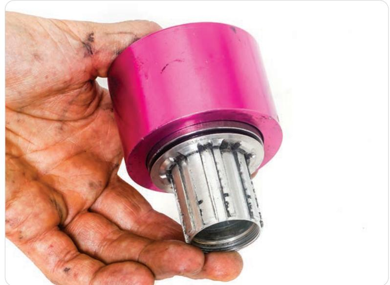
**8** Use a bushing or section of pvc to press the 61808 bearing back on. Reinstall the bearing retainer circlip.
