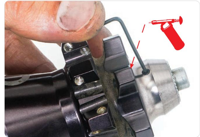
**14** Apply grease to inner bearing races as well as the bearing seats on the axle. Apply grease to the threads for the adjustable dustcover. Reapply blue loctite to the 1.5mm grub screw. Install the axle and install drive side endcap. Install adjustable dustcover until there is a small amount of lateral play.
