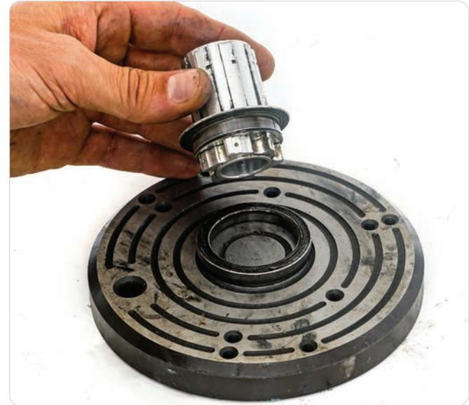
**5** Wipe any excess grease from around the pawls. Use a .050" allen to loosen the six allen bolts that hold the pawl springs in place. Wipe down the pawls and pawl pockets.
