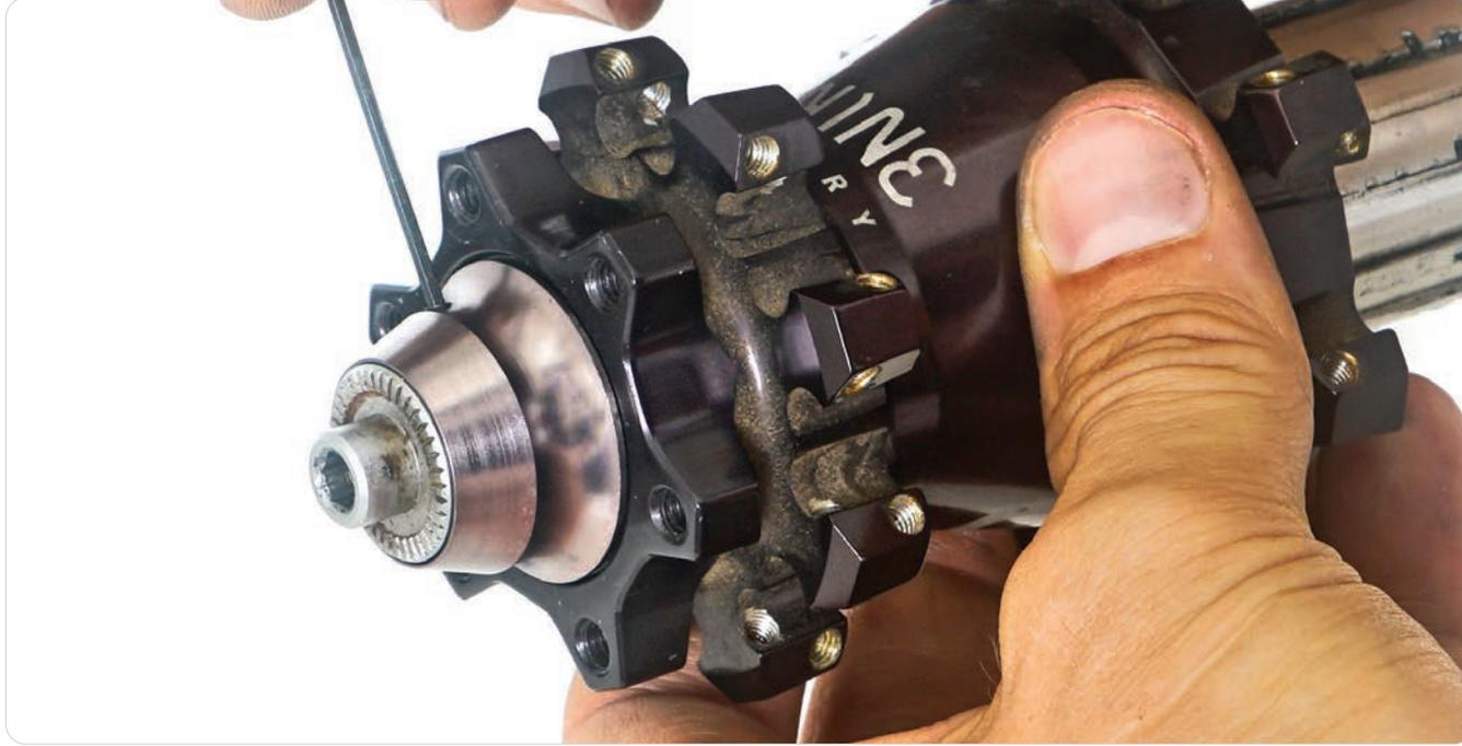
**3** The freehub body is pressed into the hubshell so it won't just pop out. To remove it you can use the axle itself (it has a machined shoulder) to help push out the freehub.
