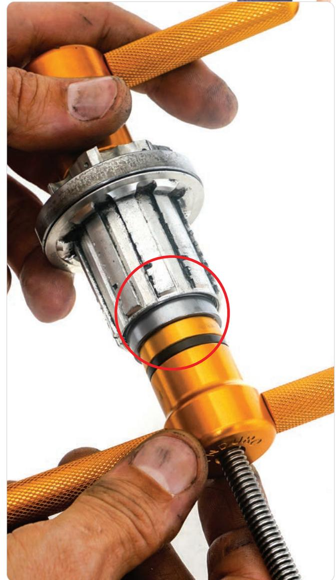
**11** Use a bushing to press the first bearing all the way into the freehub. Apply a light film of grease to the bearing spacer and push it in. Install the second bearing.
