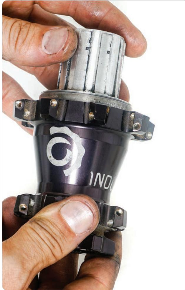
If you press it in while it's crooked, you may damage the pawl springs. Try to free wheel the freehub as you are pressing it in as that will reduce the likelihood of damaging the springs. If it feels rough, you may need to push the freehub out and start again.
