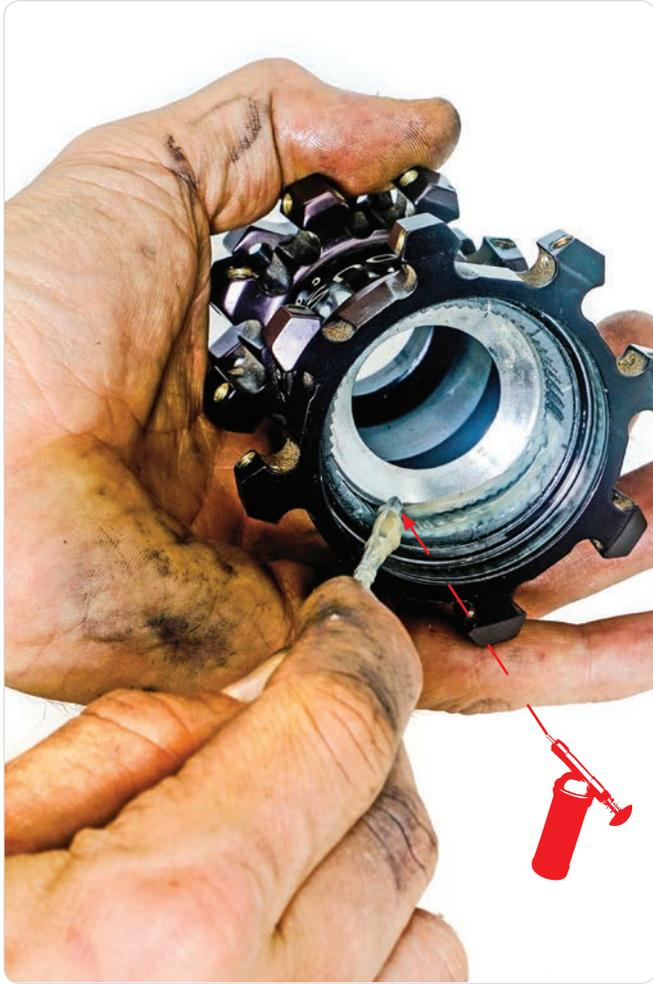
**12** Apply a layer of grease on the drive ring. gently place the freehub assembly into the hubshell to get it straight before pushing any further. ratchet the mechanism to ensure it's lined up and not crooked in the bore.
