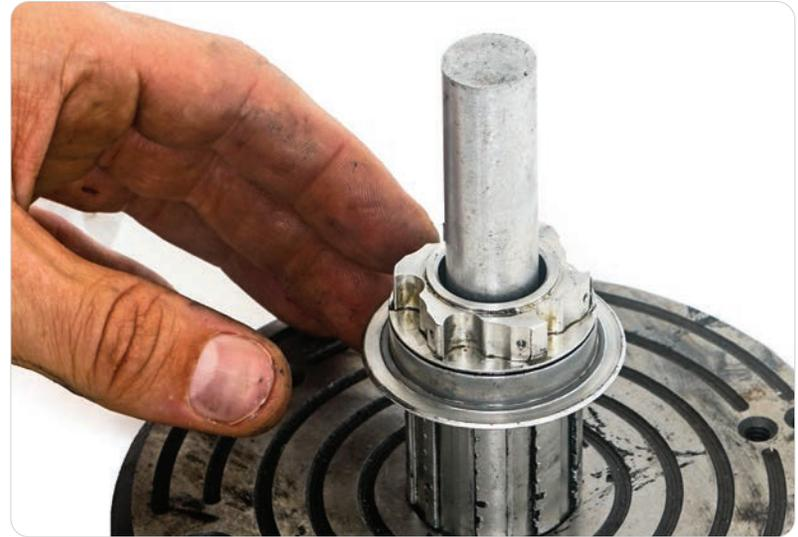
**7** Use a punch or dowel to remove the disc side 61804 bearing.
