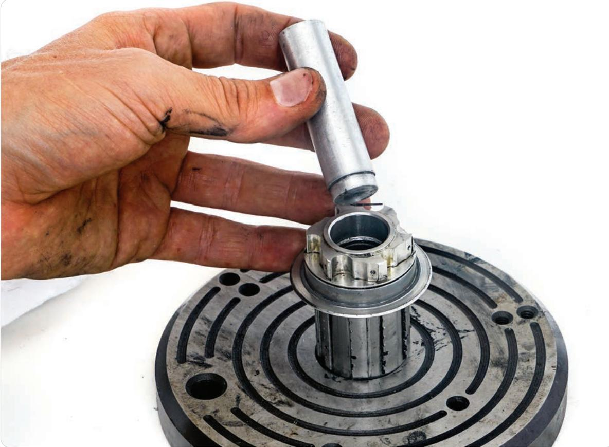
**6** To remove the two inner bearings, use a punch or dowel to catch the inner races.
